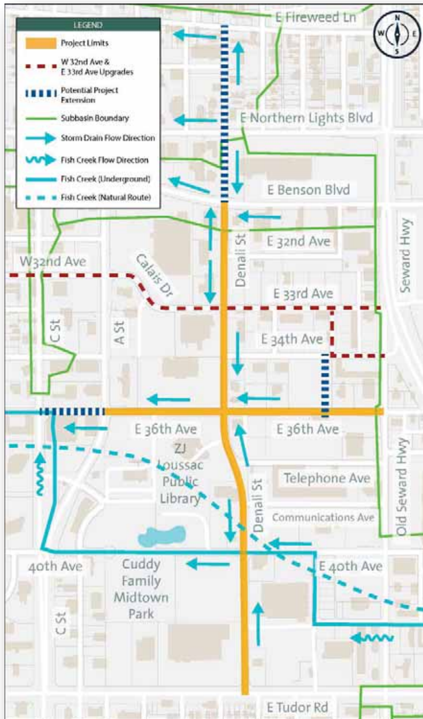
Figure 11: Existing drainage patterns
