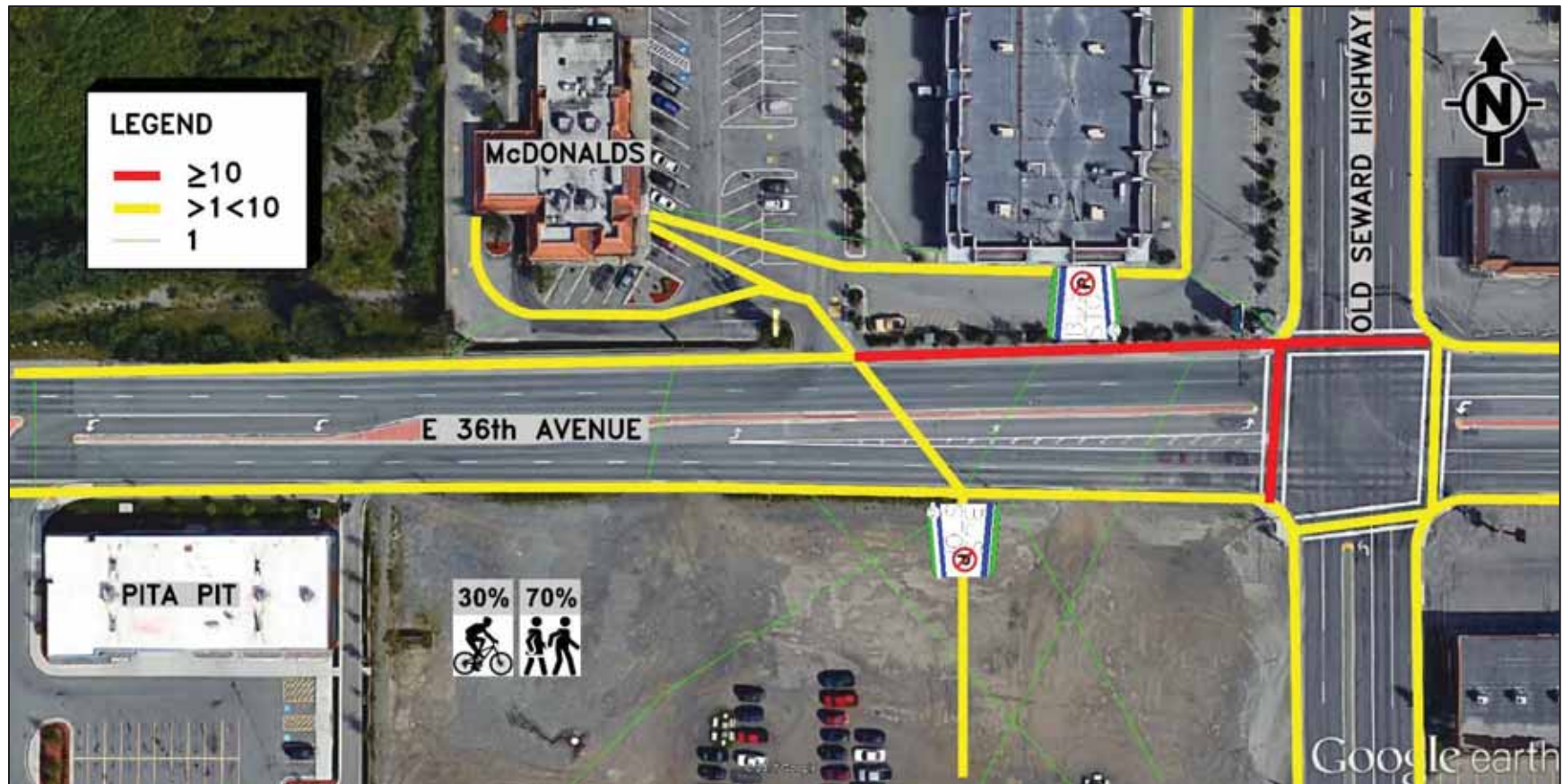
Figure 57. Ped/Bike Movements on 36th Avenue – Kuukpik Bldg to Old Seward Hwy (4:55 – 5:55 PM)
